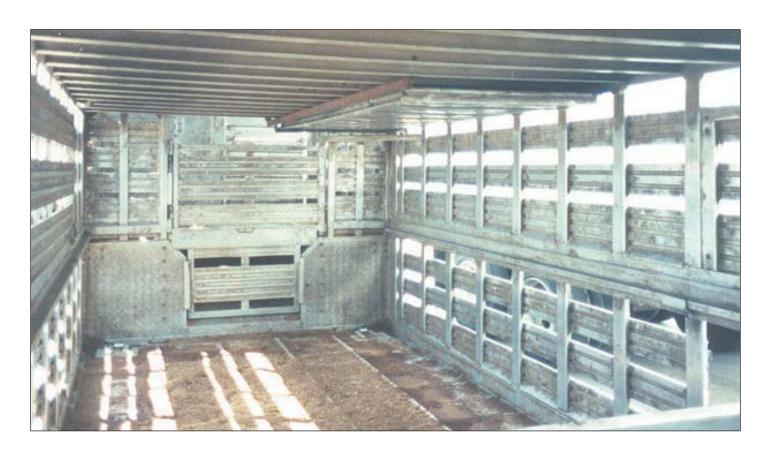
Interior view of bottom deck of double deck trailer. Besides the 3" I beams protruding below the ceiling, there is a ramp that is stored on the ceiling.
