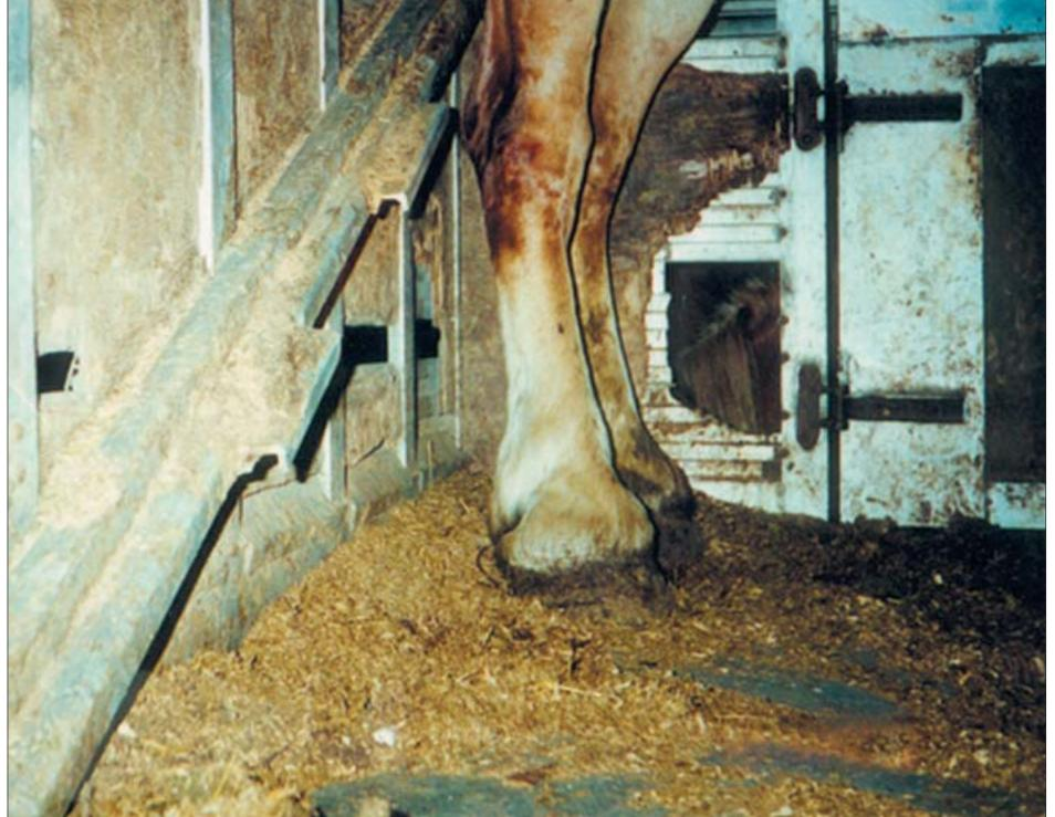
Above: Horses inside the "doghouse" area of a double decker. Note the exposed metal floor and the hole in the wall behind the horse's leg, (horses are at risk for injury if they were to kick or paw and the leg would become caught in the opening.) Aslo note the slanted, sharp metal protrusion on wall behind horse's leg, which supports the ramp to top deck when it is in the "down" position.
